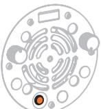
Orange | DMX Control    | Fixture is receiving DMX control signal.<br>Manual control knobs are disabled while DMX is active. |
